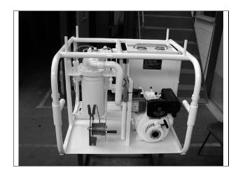
The pumpset is designed to be compact and portable by two men. The unit is engine driven and incorporates a self-priming pump; filter water separator, bulkmeter and quick disconnect couplings for the attachment of suction and delivery hoses.
